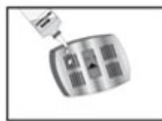
Allow the liquid to penetrate into the foam through the slots of the appliance.
