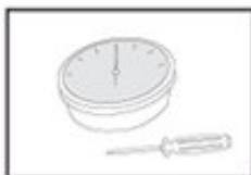
We recommend to adjust the instrument once a year. Simply wrap it up in a wet cloth for half an hour. The pointer should indicate 94-96%. If this is not the case, readjust the instrument on the back with a screwdriver.
